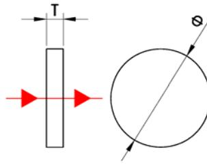
Calcium Fluoride Window is applicable for wide rang spectrum, and it is particularly useful for at 2980nm laser application.
